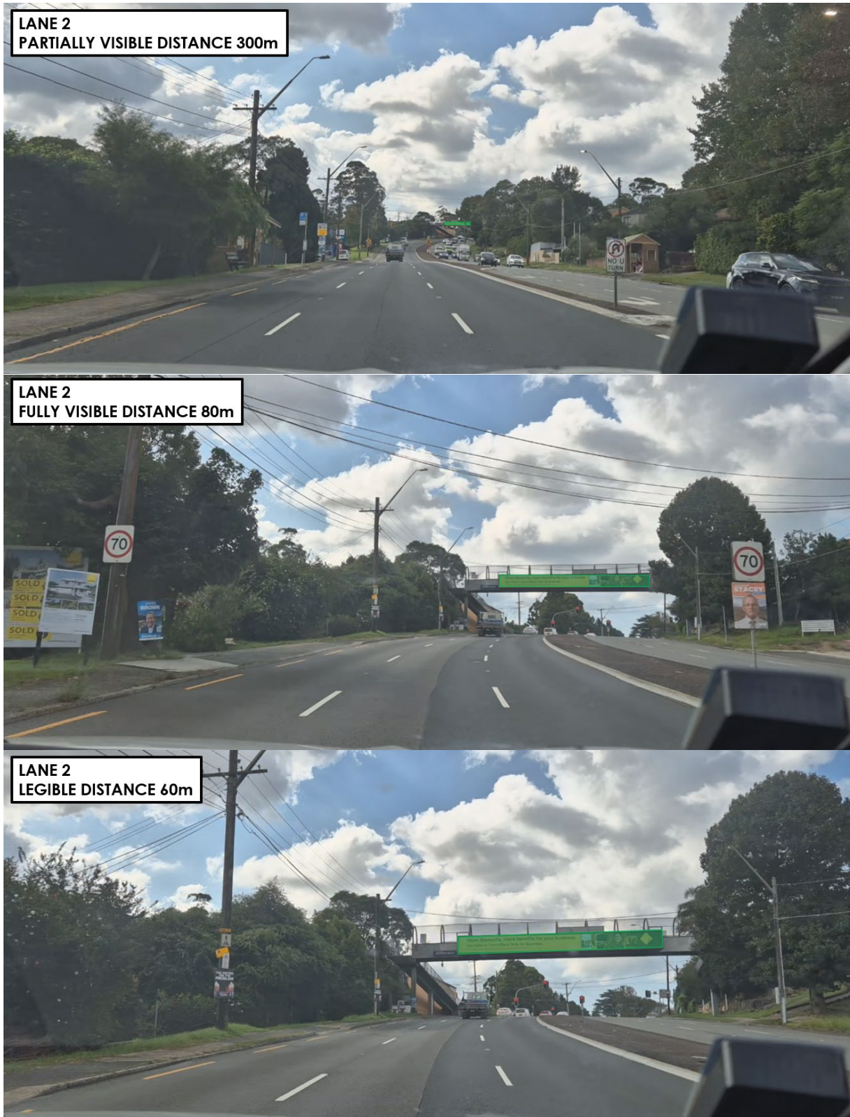
Figure 2.6: Warringah Road Eastbound Approach Sign Exposure – Lane 2
